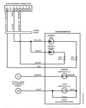
Figure 9. Keyswitch Wiring Connections
