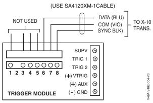
**Trigger Module Powerline Interface Connections**
