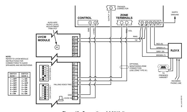
Figure 12. Connection of AAV Unit
