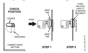
Figure 1. Installing the Cabinet Lock
