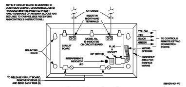
Figure 8. 5881EN RF Receiver (cover removed)
