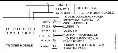
Figure 11. Trigger Module
