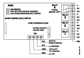
Figure 10. 4204 Connections to Control
