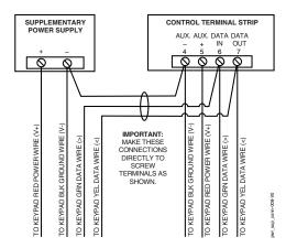
Figure 3. Using a Supplementary Power Supply
