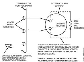
Figure 4. Sounder Wiring (Supervised)
