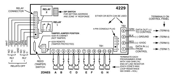
Figure 7. Wiring Connections, 4219 & 4229 (4229 shown)
