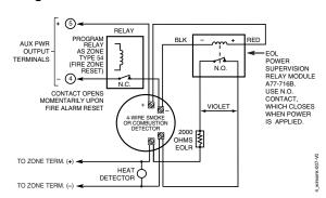
Figure 6. 4-Wire Smoke Detector Connections
